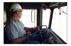
After the machine has warmed, perform steering actions with the machine parked or at a slow speed to determine if the control is responsive. Any feeling of looseness, binding, unusual noise, or stiffness in the steering control system should be checked immediately by an authorized person before the machine is put in service.
